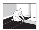
2. The underlay should be pale side down allowing a 5cm excess of underlay to run up the perimeter wall. Each roll of underlay should be closely butted-up.
