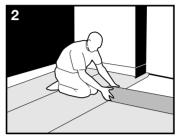
The underlay should be laid foil side up allowing a 5cm excess of underlay to run up the perimeter wall. Each roll of underlay should be closely butted-up.
