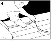
Once the Laminate or Wood flooring has been fully laid, trim the underlay around the perimeter of the room flush with the flooring, fit skirting or quadrant to finish.
