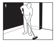
The sub-floor must be level sound, dry and free from dust, grease and other contaminants.
