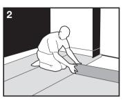
The underlay should be laid foil side up allowing a 5cm excess of underlay to run up the perimeter wall. Each roll of underlay should be closely butted-up.
